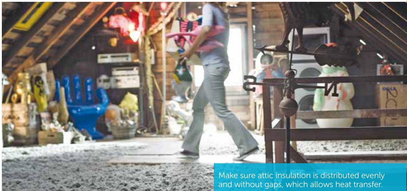
Make sure attic insulation is distributed evenly and without gaps, which allows heat transfer.
